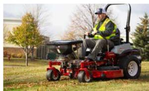
504U Receiver Mount Electric Broadcast Spreader
